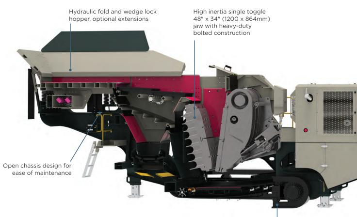
Heavy duty bolt-on tracks with smooth start/stop 3-speed system
