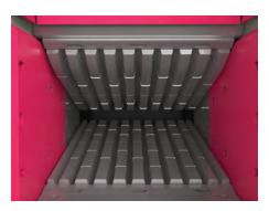
Deep 75" (1.91m) jaw chamber with single toggle design accommodates hard rock applications and large feed sizes. Also features closed side setting adjustment with hydraulic wedges.
