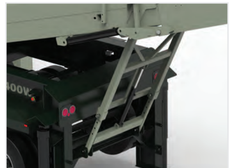
Hydraulic height adjustment on discharge conveyor.
