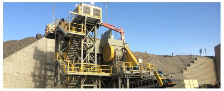
This primary crushing station is designed for heavy-duty and high production applications. With it handling 100-ton trucks this plant is capable of 1800-2200tph. Lippmann designs customer primary stations that will fit their needs and demands. Keeping safety in mind, Lippmann has designed these plants with plenty of clearance to easily maintain this large equipment and provide optimum uptime for the customer by allowing material to flow freely.
