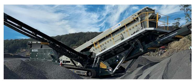
The most advanced and innovative 20'x5' portable vibratory screening plant today is the L520s-t. Featuring adjustable screen box angles allowing adaptability to a wide range of material applications including quarrying, mining, sand and gravel, coal screening, topsoil and woodchip. With the highest-grade specifications and component parts, and offering a triple deck makes this screener a top choice for high productivity, quality and value.
