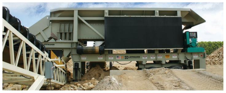
A completely self-contained or electric, high production screening and scalping unit that offers a full 62" wide by 24' long vibrating grizzly feeder. Lippmann's larger grizzly area offers 30 percent more capacity and maximum throughput. Smaller rock separates easily, so your plant can run at higher speeds to optimally produce the engineered rip-rap you need.
