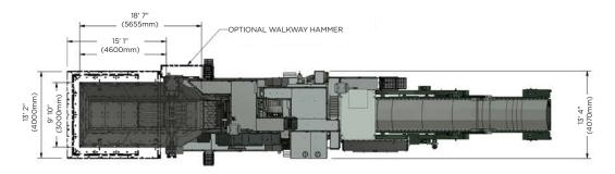
12' 0" - 14' 7" (3600 - 4450mm) discharge height with 55" (1397mm) belt width
