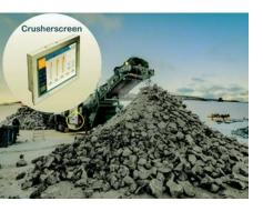
Standard telematic control system delivers machine data to a central dashboard for convenient monitoring of belt scales, automation system, generator/engine, and alarm logs and diagnostics.
