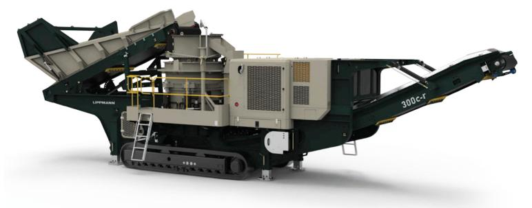
The ultimate in versatility, the heavy duty 300c-tr tracked cone crusher features an innovative material flow that maximizes capacity and throughput while delivering a consistently high-quality product. The recirculating system creates the finished product with just one crusher. The tracks enhance the job site mobility of this crusher.
