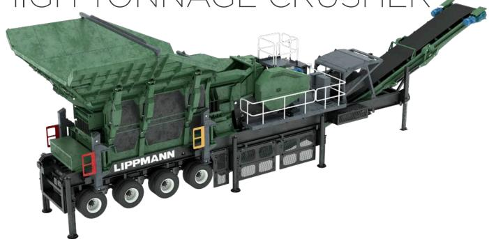
The 34x47 wheeled plant has been developed to be a high tonnage crusher with both the ease of maintenance and transportability. The 34" gape allows you to feed a 27.5" rock with ease. The jaw also features an opposing wedge design that allows the producer to make adjustments easily and safely.
