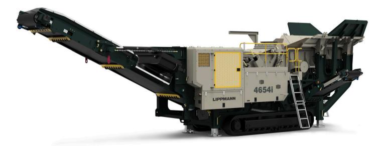
Heavy duty track mounted crusher with following features: 1200mm (48") diameter x 1350mm (53") wide impactor, 510 Hp (380 kW) Volvo D13 Stage V engine / 516 Hp C13 CAT LRC / 536 Hp C13 CAT, tracked, integrated hydraulic folding hopper, integrated hydraulic folding stockpiling conveyors, I-beam plate fabricated chassis construction, open chassis design for ease of maintenance, fast setup time, and vibrating feeder under crusher discharge.
