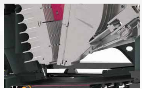
The large gap between crusher discharge and main conveyor belt, paired with wide main and side conveyors result in an optimized material flow.
